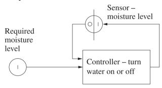
Technical problems that can arise from a continuous monitoring system, such as this one, are overdamping and under damping. Over and under damping in this scenario would result from the level of drainage from the pot plants and the rate at which water is added.
